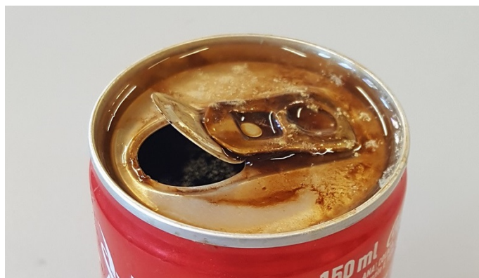
Figure 2. Failure occurring to a mini-can incubated in contact with the beverage, as to simulate the product spilled from a damaged adjacent can.
