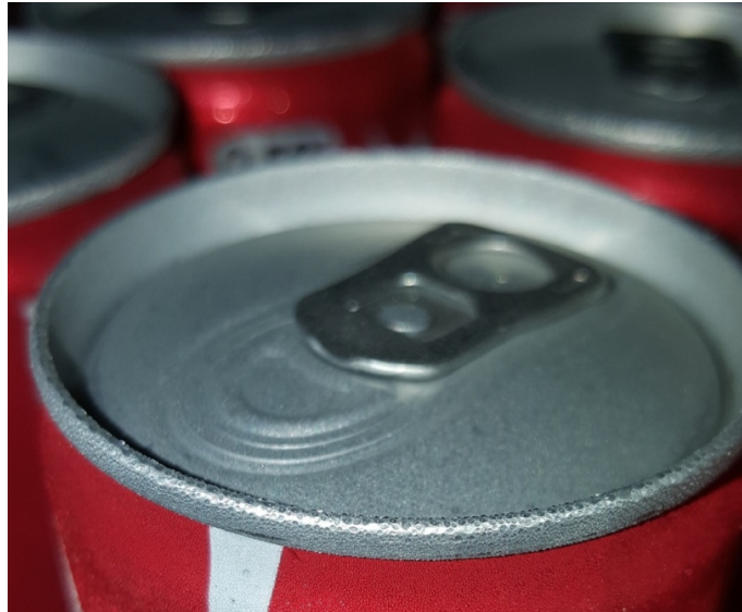
Figure 1. Condensation occurring on the can surface. After filling with the cold beverage, cans must be warmed above the dew point to prevent “can sweating”.
