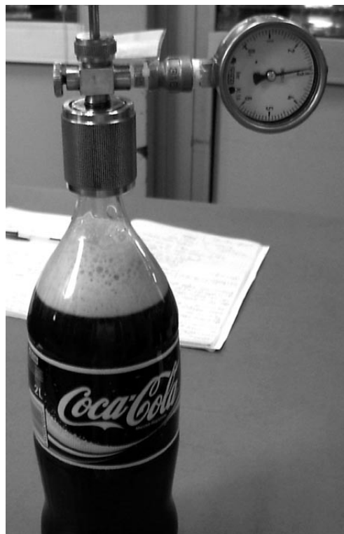
Fig. 1. Zahm and Nagel piercing device for CO 2 retention test.
