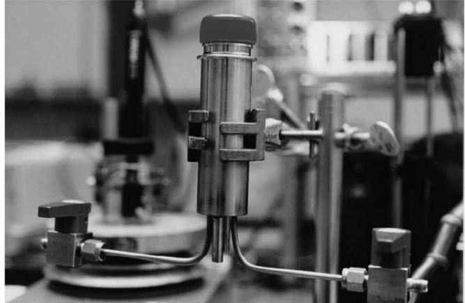
Fig. 3. Ready-use-tool to measure oxygen permeation and adsorption by scavengers in closed containers.
