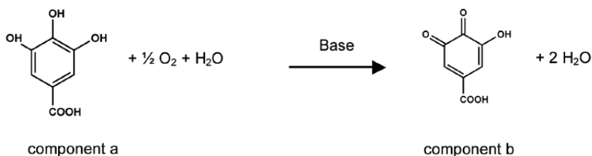
Eq. 1. Mechanism of the reduction of oxygen by gallic acid (component a) in presence of an alkaline milieu; component b: 5-hydroxy-3,4-dioxo-1,5-cyclohexandien-1-carboxylic acid.
